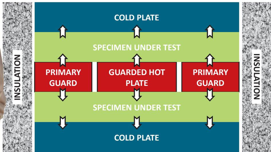
Two identical specimens are needed for one test.
